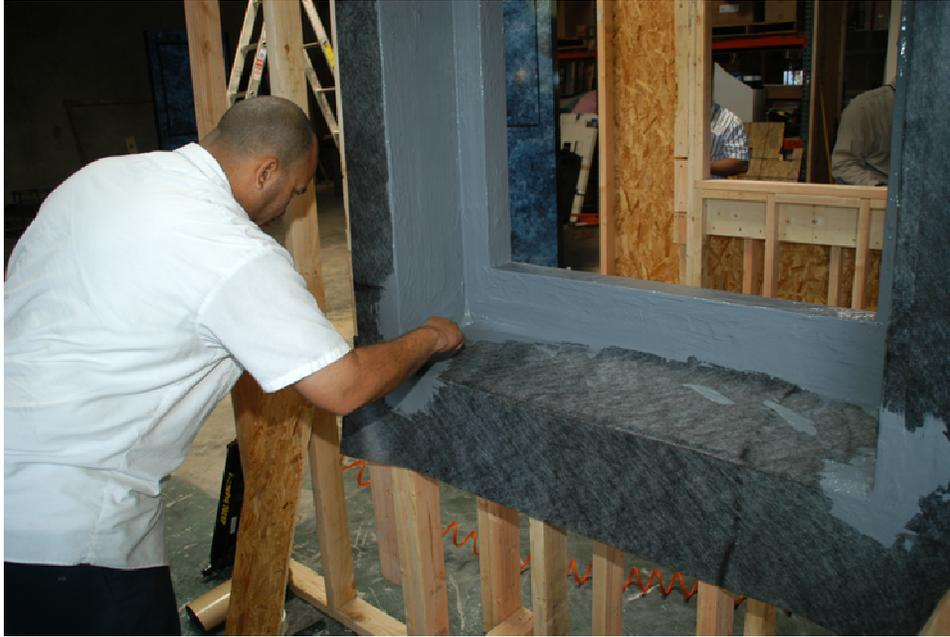
**New membrane prototypes being tested in 2007 in our test facility.**
